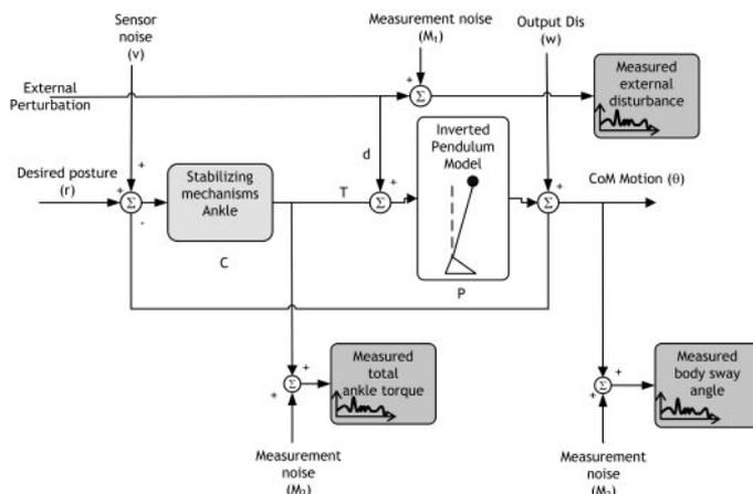
FIG. 1. A simple model of balance control.
