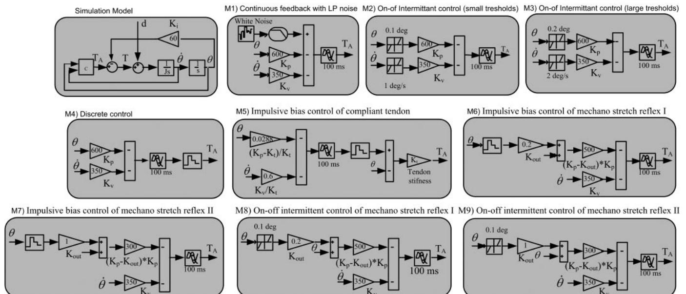
FIG. 2. General simulation model of balance control (*top left*) and 9 different models (*M1–M9*) representing the stabilizing mechanism as used to evaluate the experimental data.
