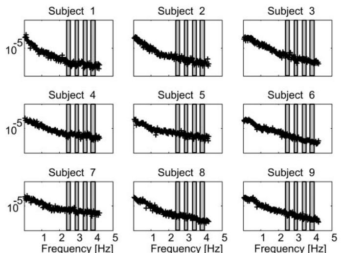
FIG. 4. The remnants of the ankle torque for EO8. Shaded areas show the frequencies where the perturbation signal contained zero power.
